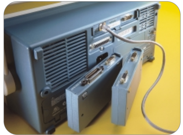
► Figure 55. A TDS3000 Series oscilloscope provides a wide array of communications interfaces, such as a standard Centronics port and optional Ethernet/RS-232, GPIB/RS-232, and VGA/RS-232 modules.
